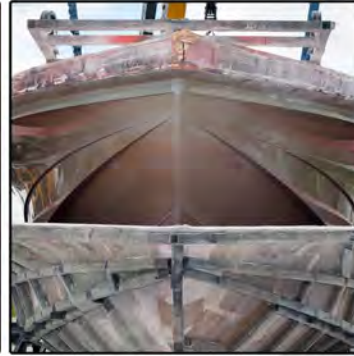
Duratec Primers can be top-coated with epoxy primers. The Vinyl Ester Primer can be directly top coated with urethanes.
